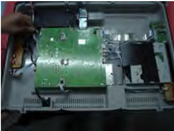
7. Remove video main board: unplug flat cable on video main board firstly.
