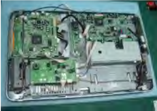
15. Arrange flat cable and check technique inside machine.
