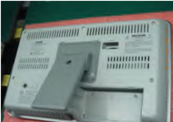
17. Use screw to fix rear cover and install support bracket.
