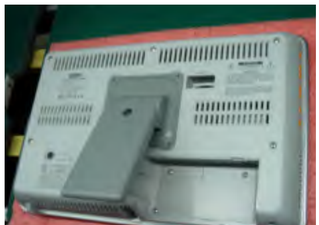
18. Use screw to fix support bracket and machine assembly finishes.
