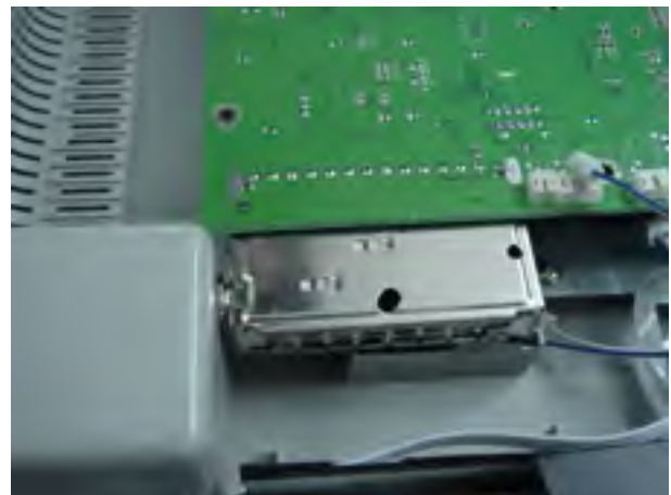
10. Take out video main board. Please note that tuner of the video main board still locks on rear casing, so take out according to arrow direction.
