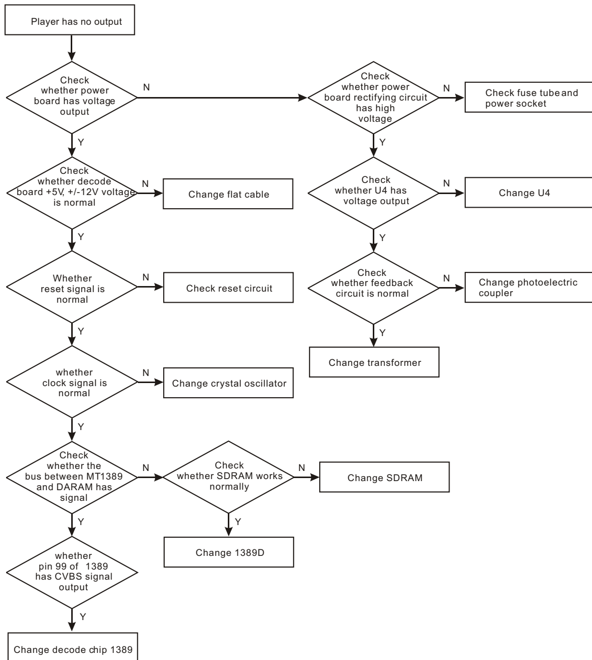
Figure 3.3.2.1 Troubleshooting flow chart for “Player has no output”
