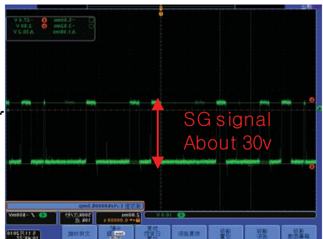
< Waveform of GR and SG signal >
