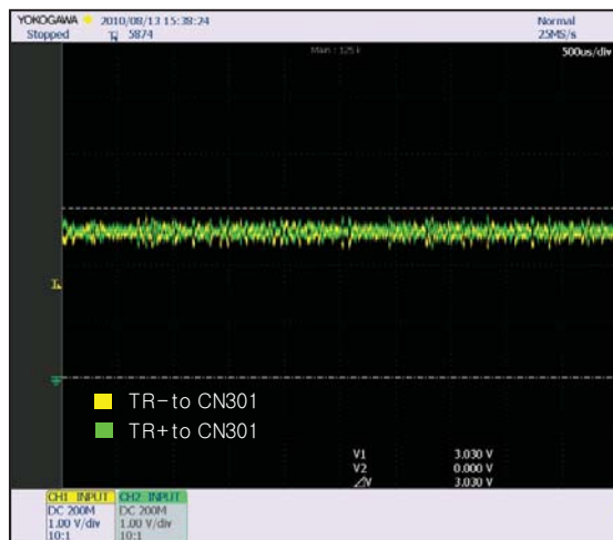
< Waveform of TR± for driving TRACKING actuator >
