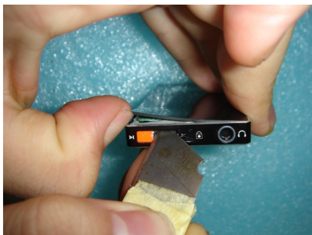
2. Use sharp blade gently from button hole to prize glass of front casing;
