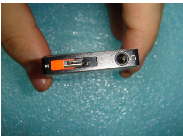
1. Use forceps to take out power on/off core-start switch;
