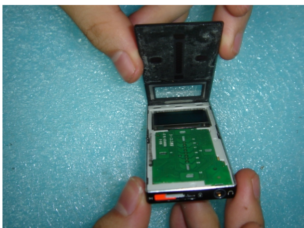
4. Peel off front casing glass from middle casing to reveal decode board;
