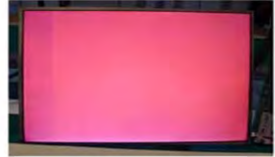
Vertical Block Source TAB IC Defect
