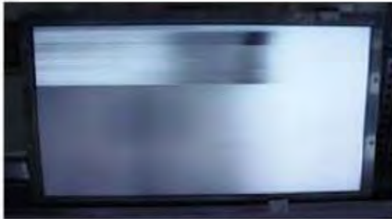
Horizontal Block Gate TAB IC Defect
