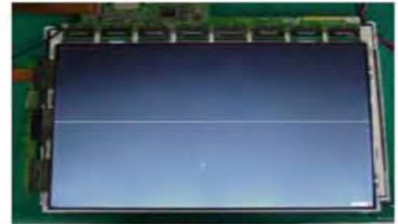
Horizontal line Gate TAB IC Defect
