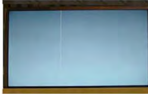
Vertical Line Source TAB IC Defect
