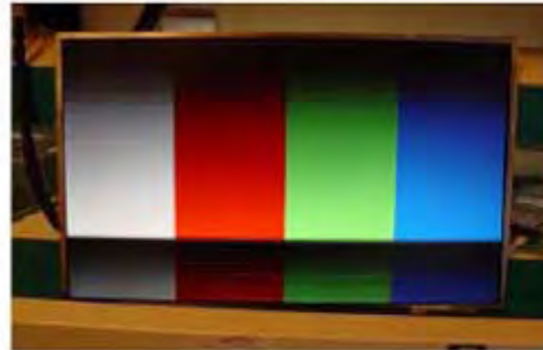
Horizontal Block Gate TAB IC Defect
