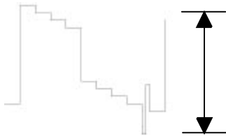
Fig. 19 Signal Y Pins 1 of Connector P0YU ; 1.3Vpp
