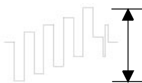
Fig. 20 Signal Pb Pin 3 of Connector P0YU ; 1Vpp
