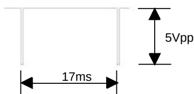
Fig. 18 Vertical Sync Signals TP5854
