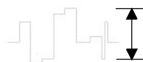
Fig. 21 Signal Pr Pin 5 of Connector P0YU ; 1Vpp
