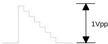
Fig. 14 Signal RGB Pins 1, 3, and 5 of connector P0PC
