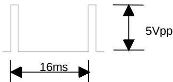
Fig. 5 Pins 9 and 12 of Connector P0YU (vertical sync signals)
