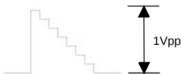
Fig. 14 Signal RGB Pins 1, 3, and 5 of connector P0PC
